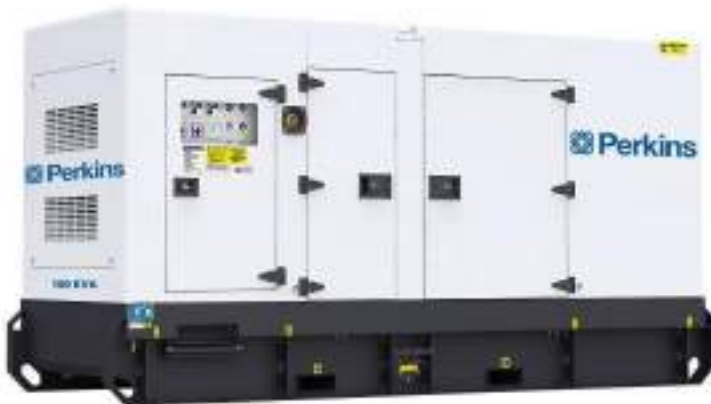
100 kVA, 3-Phase Silent Diesel Standby Generator Set complete with 200 A 4-Pole ATS, acoustic canopy, integral fuel tank, accessories, installation, testing and commissioning.
